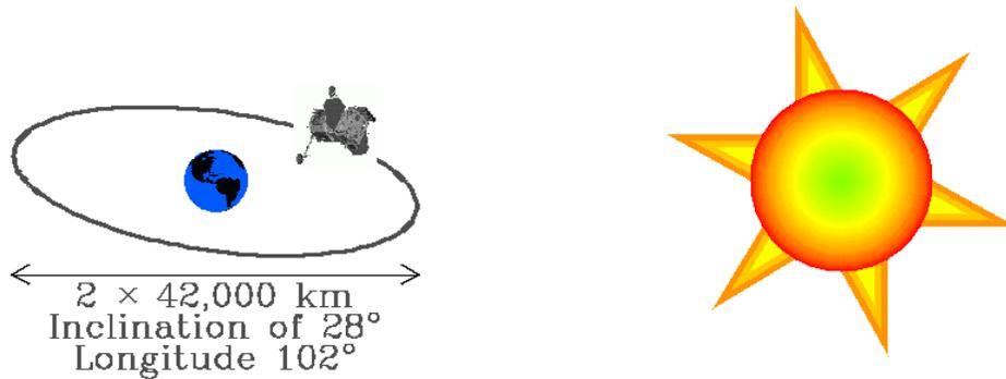
**Figure 2.1: Simplified Orbital Configuration of SDO. The orbital radius is scaled to the radius of the Earth, the distance and size of the Sun are not to scale.**
