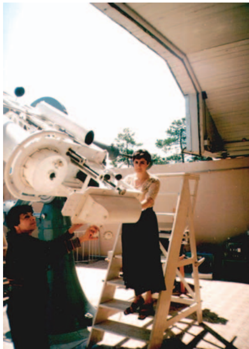
Fig. 50. The Lyot-type extra-eclipsing coronagraph ( D = 12\text{ cm} , F = 300\text{ cm} ).
