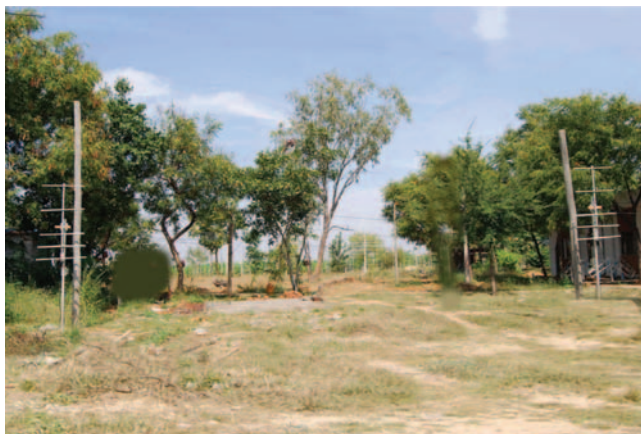
Fig. 23. Two-element radio interferometer antenna system (the antennas in the foreground) fabricated at the Gauribidanur observatory for donation to colleges/universities in India as a part of the IHY-PO program.
